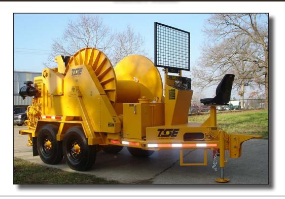
The DP100 is a heavy duty drum puller designed for transmission line stringing in the 3500-4500 daN (8,000-10,000 lb) range. Powered by a 123 kW (165 hp) diesel engine with twin hydrostatic transmissions, the unit provides continuous, infinitely variable speed, torque and directional control within the performance parameters.
